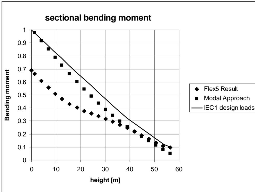
**Fig. 5:** Results of the different methods compared with the IEC1 design tower loads. Results are given relative to the design moment at the tower base
