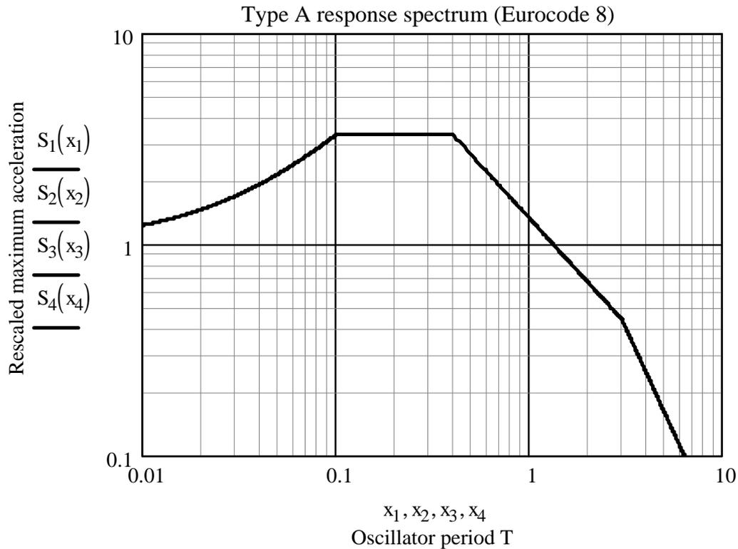
**Fig. 2** Response spectrum for SDOF oscillator according to Eurocode 8 [4] for subsoil class A (firm ground).
