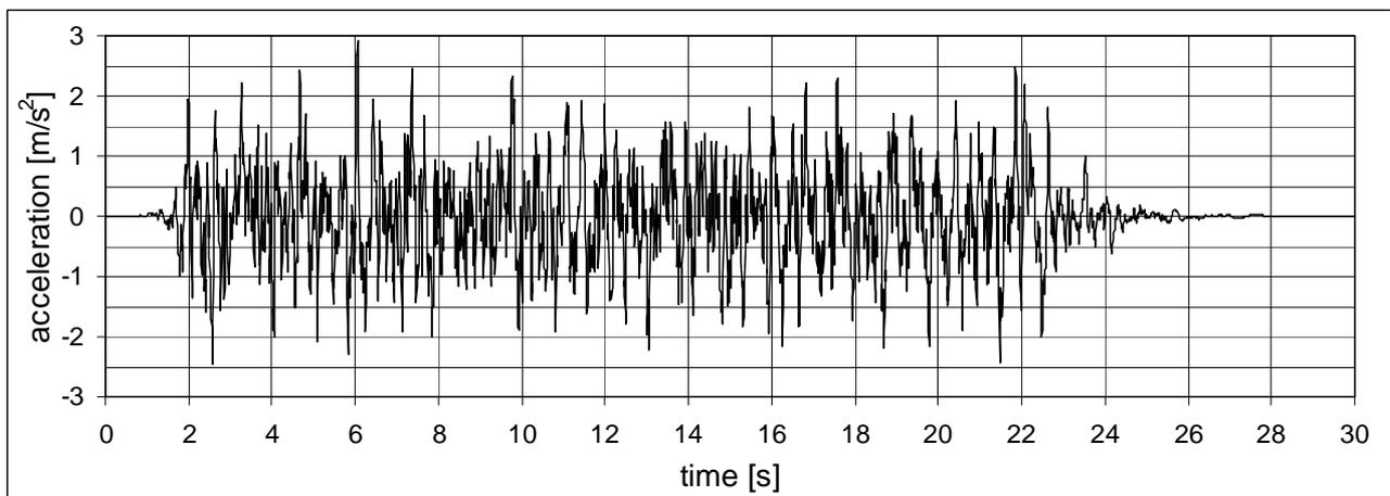
**Fig. 3:** Typical accelerogram applied in the load cases with a peak acceleration of 0.3 g or 2.94 m/s<sup>2</sup>.
