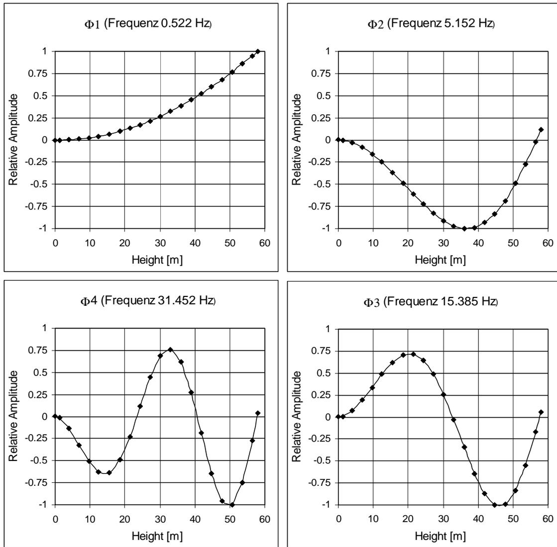
**Fig. 1:** Normal modes and corresponding frequencies. The modes are normalized such that the maximum modulus of the amplitude is 1.
