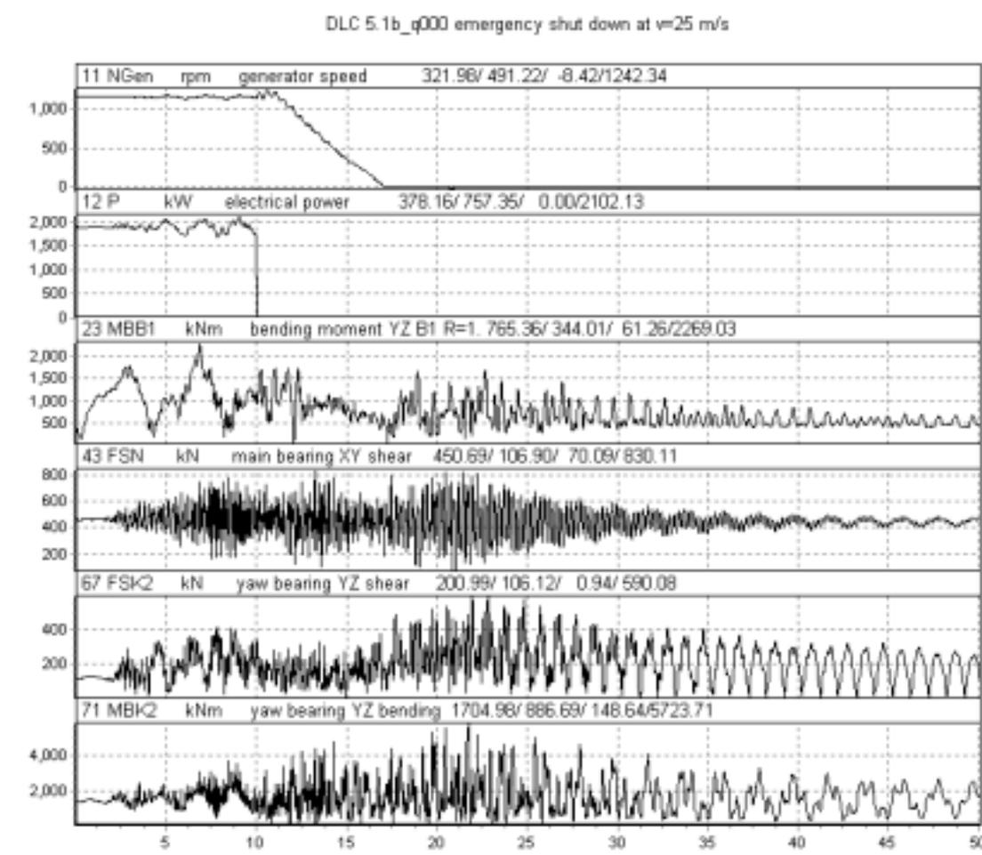
**Fig. 4:** Selected time series that give an impression of the behavior of the turbine during an earthquake. They are taken from the load case with epicenter in 0°-direction. The first two plots show rotational speed and power. The corresponding ground acceleration was illustrated in Fig.1. The earthquake starts at zero, and the shut down takes place after 10 seconds. The effects of the earthquake can be clearly seen in the resulting sectional loads shown in the plots.
