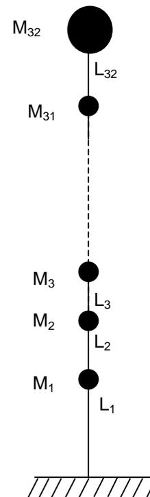
**Table 1:** System of lumped masses and flexible rods representing the wind turbine, where  $H_i$  and  $M_i$  are height and mass of  $i$ -th element,  $L_i$  and  $E^*I_i$  the length and bending stiffness of the  $i$ -th rod.
